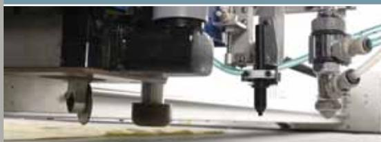
All Eastman automated cutting systems feature individually aligned and calibrated tool spindles which may be fitted with any combination of different sized rotary blades, different angles of straight knife blades, various shaped notches and various sized punches. ....[p.7]
