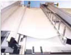
Eastman's EasiPull™ increases throughput by streamlining spreading; it is a perfect attachment to a longer or wider cutting table. EasiPull™ automatically pulls material from the end of the table to the exact length needed for each cut.
