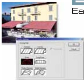
Eastman Tent and Awning Suite, ETADS™, is specially designed for the needs of tent and awning manufacturers. ETADS™ is an AutoCAD based tool that automates the very tedious task of turning a three dimensional wireframe to a two dimensional form that can be cut with ease.
