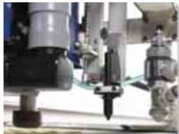
Eastman automated cutting systems feature individually aligned and calibrated tool holders which may be fitted with any combination of different sized rotary blades, different angles of straight knife blades, various shaped notches, and many sized punches. All tool heads include a pneumatic pen/marker holder and the optional EasiMark™ airbrush marking system.
