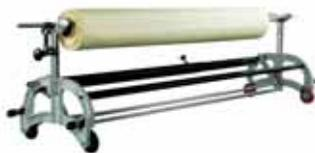
Eastman's Expandable Roll Carrier is capable of spreading various width materials using one system. The Expandable is an ideal first machine or an emergency machine for cutting rooms with motorized spreaders. The manual edge control and lifters guide the material onto the table as the operator spreads it along the cutting table.
