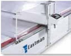
Eastman's EasiHold™ dynamic vacuum compressor is an integral part of the Eagle-FC Fiber Cutter System, allowing users to cut lofted material, such as fiberfill and foam, with unparalleled speed and ease. EasiHold's™ vacuum compressor holds down porous and thick fabrics for cutting using a tough transparent plastic overlay. The plastic overlay curtain is never cut, eliminating consumable waste.
