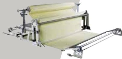
The Pacemaker is Eastman's top-of-the-line manual spreading device. It can be used for either face-up or face-to-face operations. It is light weight, easy to use, reliable, strong, and durable. Its ease of operation coupled with its many features for increasing productivity make it an economical solution. The standard Pacemaker comes with end catchers, which automatically fold and clamp the fabric at each end of the spread.
